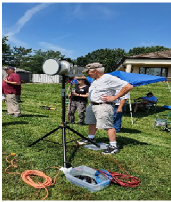
Chris W3CMP with the 10" Lens Horn, getting ready for 24 GHz MDS - WA3NUF
