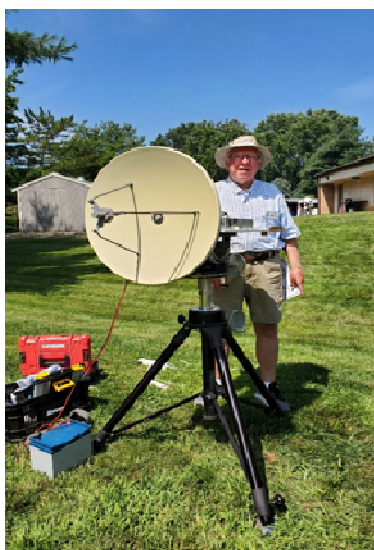
Al W9KXI 24" DSE Dish ready for the 10 GHz MDS. Photo by WA3NUF
