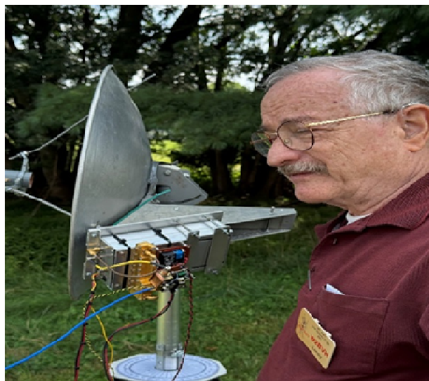
Lenny W2BVH contemplating adjusting the feed horn spacing to optimize signal strength on his new set-up – the Tune Up to improve his MDS. AA2SD
